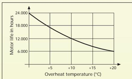
As one can see, a 10°C increase in temperature reduces the useful life of the motor by half.
