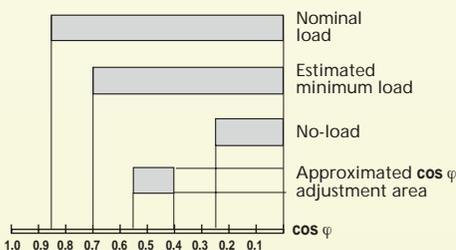
If the above mentioned  $\cos \varphi$  values are unknown, the underload trip setting can be made in the following way:
